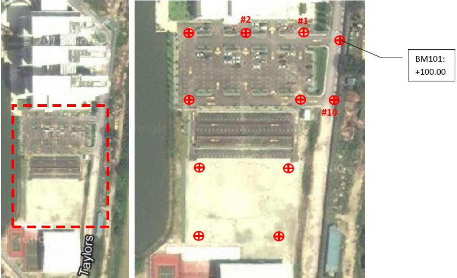
The picture attached above show the area and the location of points of the leveling at Taylor's University Lakeside Campus, Car Park Area.
